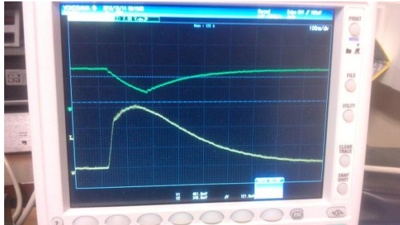
Fig. (5). The PMT signal was amplified and the pulse from the discriminator is shown as the yellow and green lines respectively on the oscilloscope
