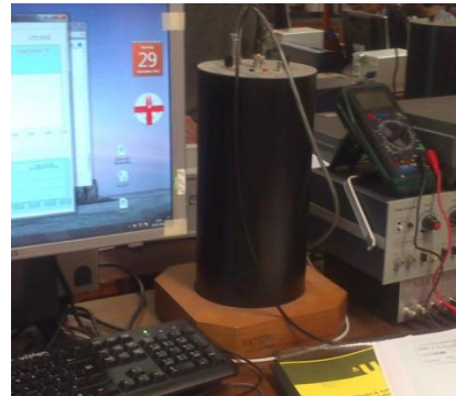
Fig. (3) The black anodized aluminium cylinder which houses the PMT and scintillator.
