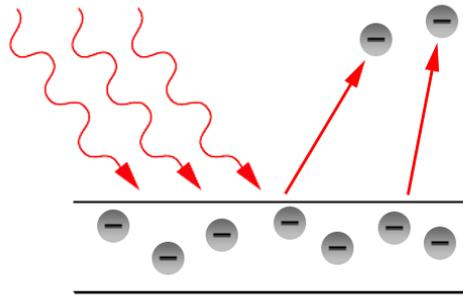
Figure 2 - The Photoelectric Effect
