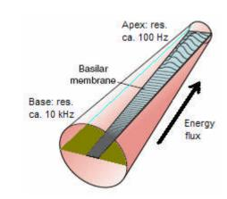
Simulation treats a continuous transmission line (resonance f=10 kHz to 100 Hz) as below. The time constant for passive amplitude decay is generally set uniformly at 2 ms (r=0.5 ms<sup>-1</sup>).
