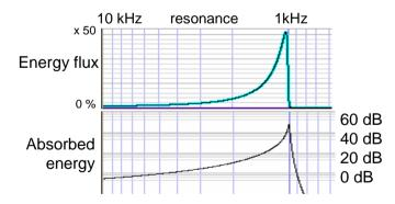
Negative feedback (stiffness at low freq x 4.1 everywhere), with uniform 3dB roll-off at 100 Hz (1st order filter, time constant 1.5 ms). Stimulus: 1 kHz. Viscosity x2 to reduce sharpness of the activation peak. There is a ca.50-fold (17 dB) increase in energy flux and ca. 40dB increase of peak sensitivity compared with the passive model.
