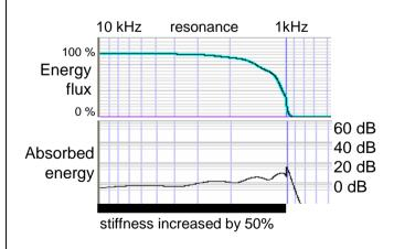
Note that the abrupt change of stiffness here causes standing waves by reflection.
