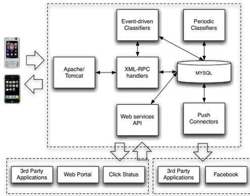
Figure 3: Software architecture of the CenceMe backend.
