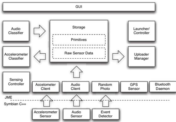
Figure 1: Architecture of the CenceMe phone software.
