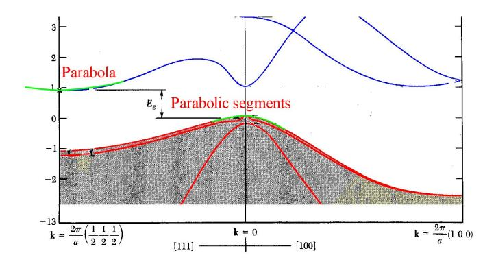
In a region close to the maxima and minima, a parabolic approximation can be accurate. From equation 1
