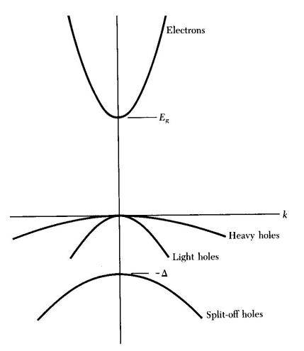
Note that the top of the valence band is often degenerate, with heavy and light holes and a split-off hole band arising from spin-orbit coupling.
