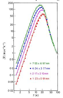
Thermal conductivity of LiF plotted as  $\kappa/T^3$  as function of temperature for low temperature.
