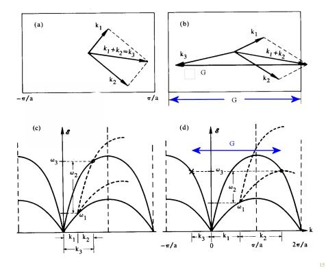
If the two initial wavevectors add to a new wavevector which is outside the Brillouin zone, they give a new wave with a group velocity in the opposite direction. Usually, subtract G, a reciprocal lattice vector, to get back into the Brillouin zone:
