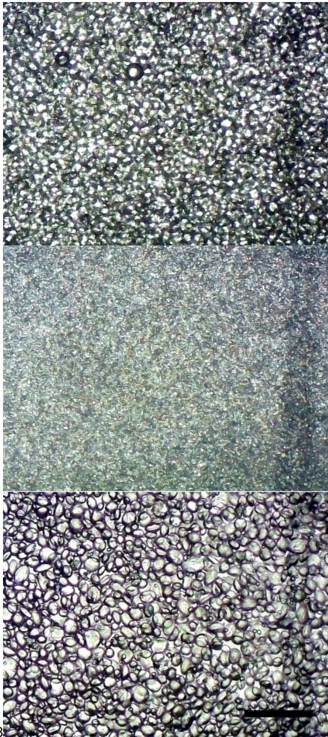
429Figure 7 – Microscopy of starch from different sources. Top to bottom – 50% HES in water; 43050% starch from rice in water; 50% starch from wheat in water. Scale bar is 100 \mu\text{m} . Images 431were taken in a static system, where no shear was applied.
