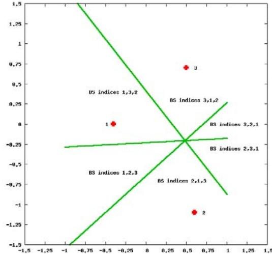
**Figure 7:** Using three BSs with the strongest signal
