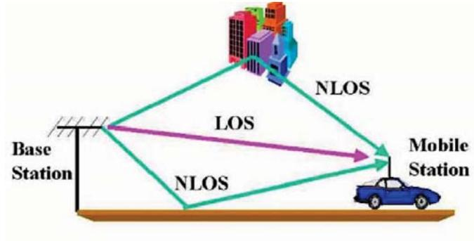
**Figure 2:** A signal from a base station can travel either by a line-of-sight path (LOS) or by non-line-of-sight (NLOS) paths
