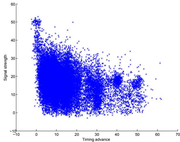
**Figure 3:** Signal strengths of the serving BS plotted against the timing advance
