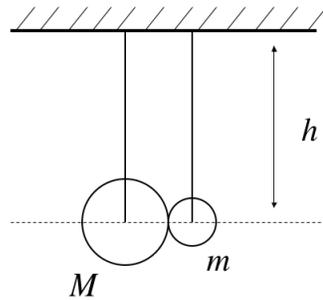
Consider the version of Newton's cradle shown: two masses,  $m, M$  hang vertically so that their centre of masses are vertically below their supports and so that they are just touching. The mass  $m$  is pulled upwards (so that the string remains taut) to a height  $h/2$  from the lowest point and released. If the coefficient of restitution between the balls is  $e = m/M$  find the speed of the mass  $m$  after the first and second impacts.
