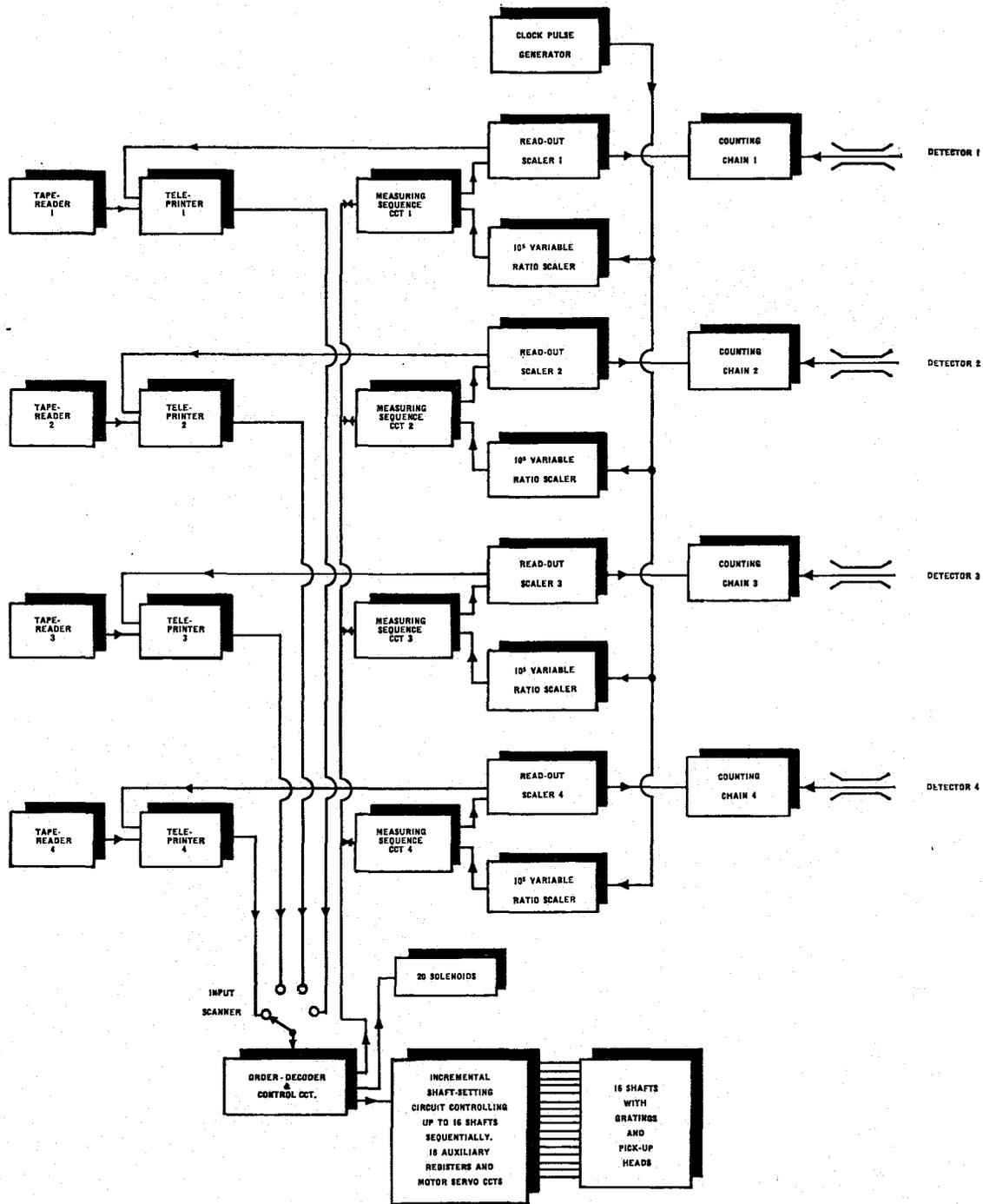
Fig. 3—Block schematic circuit diagram for a four-diffractometer installation
