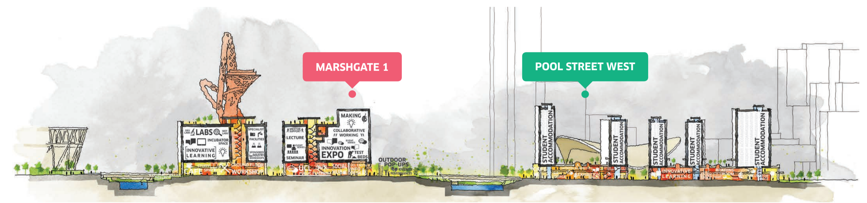
Masterplan: Illustrative view of UCL East in section from the south (the yellow and red tones represent the active street levels of the 'Fluid Zone')
