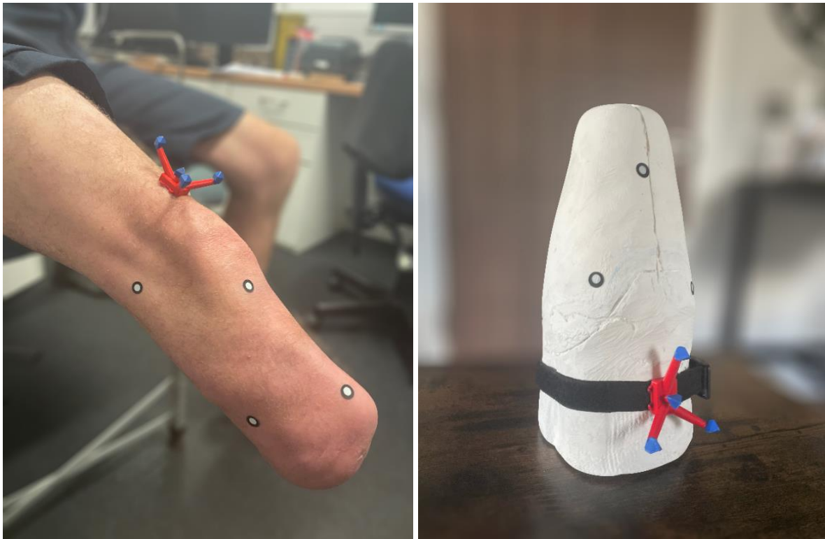
Figure 1. a) Transtibial limb of Participant C during scanning. Tracking stickers are placed randomly around the limb, enough such that at least two are visible from any angle, and the scaling object is placed with double-sided tape around the bony prominence on the knee to minimise movement during scanning; b) Transtibial model in the home environment with natural lighting. Tracking stickers are placed around the limb, and the scaling object is connected to the limb with a Velcro strap to improve adhesion.
