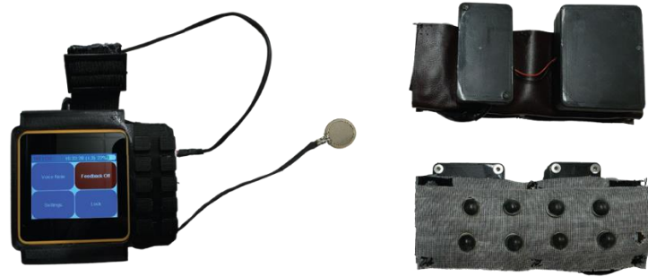
Figure 1 Sensor Control Unit (left), Vibration Feedback Device (right). The vibration feedback device shown is a version that is designed to be placed on a prosthesis harness for body-powered prostheses and high-level powered prostheses.
