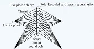
2. A pole can be supported by thin fibres that are anchored in opposite directions. The point of failure is not a local point due to multiple threads and therefore the pole can be thin.
