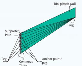
4. The fibres holding the structure can also stop the bio-plastic from deforming and also create a surface.
