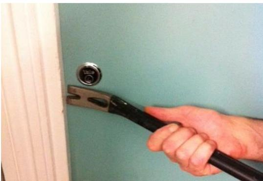
If you have a door that will not open from the outside you can try applying sideways pressure to the key (try various angles). Make sure that any other locks or latches on the door are open (handles pushed down).
