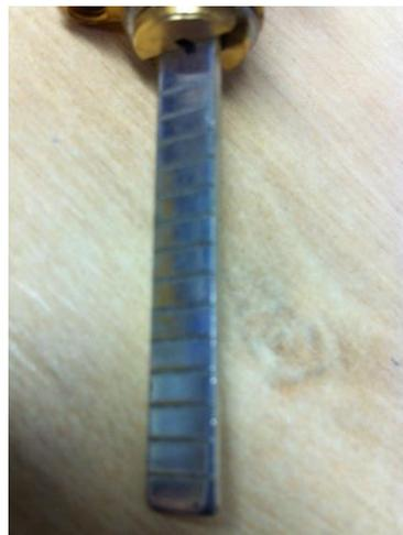
Find a replacement cylinder/barrel cut the barrel tail (using a hacksaw or large cutters) to the desired length (factor in door width and enough in order to engage with the lock assembly), as mentioned earlier some tails have grooves to assist with measurement and cutting. Screw the cylinder back on to the door through the lock bracket (opposite of step three above).
