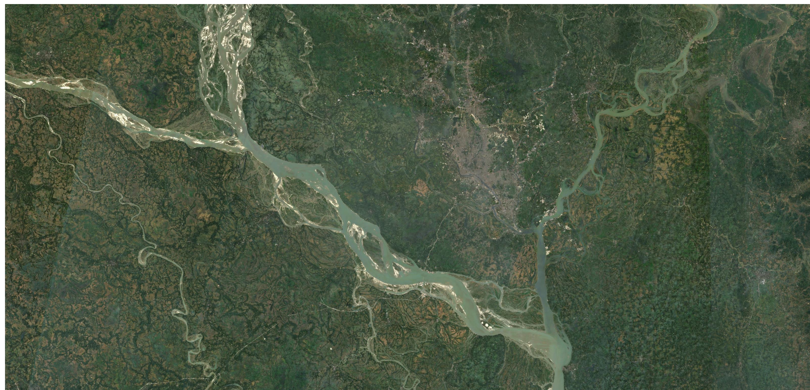
Cloud free composite generated using all Sentinel-2 images from January to March 2020. Image is shown in a true-colour composite (red, green, blue) RGB. The image was used as part of the land cover classification framework to capture seasonal changes in vegetation.
