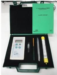
The formaldemeter htV can precisely measure formaldehyde concentrations in parts per million (ppm) and mg/m<sup>3</sup> over a wide range of temperature and humidity. Sampling methods include a 10ml snatch-sample of air taken by internal pump at a frequency of 1 minute in normal IAQ conditions.
