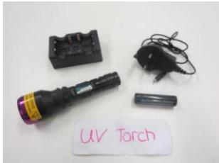
Portable UV torch allows detecting different materials (e.g. varnishes on paintings) depending on its absorption of UV radiation.
