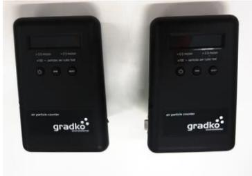
Detection of airborne particulates including dust. The instrument is simple to use and can be mains or battery operated. Calibration range PM1.0 and PM5.0; Air Particle Counter DC1700: calibration range 0.5  $\mu\text{M}$  /2.5  $\mu\text{M}$ .
