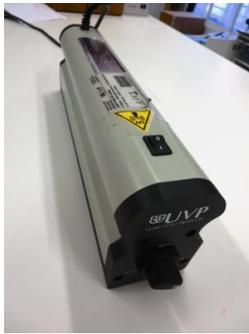
Portable UV lamps allows detecting different materials (e.g. varnishes on paintings) depending on its absorption of UV radiation. UVP 3UV lamp.
