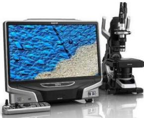
All-in-one microscope that incorporates observation, instant high-resolution fully-focused image capture, and measurement capabilities. It was designed to overcome the limitations of traditional optical microscopes by providing large depth-of-field imaging and integrated 2D/3D measurement in a system.
