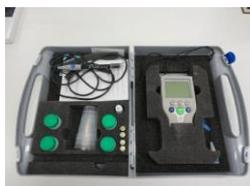
The instrument can be used to measure acidity or alkalinity of a solution - also know as pH. Mettler Toledo.
