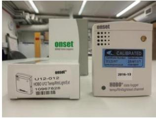
HOBO Data Loggers - U12-012, U23-001, UX100-011; iButtons. Monitoring of relative humidity, temperature and light in different environments (also with highly humid). iButtons allow measurements in small spaces such as boxes and inside objects.
