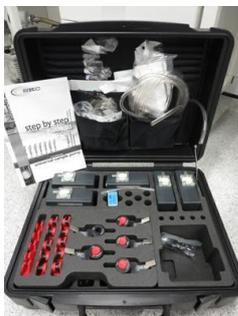
The Universal Air Sampling Pump is suitable for particulate and vapour sampling and has both an inlet and an exhaust port to make bag sampling a breeze. ATEX approved and capable of flows between 5 and 4000 ml/min without requiring an adaptor. Universal Deluxe five pump Combined kit (224-PCMTX8K5C). SKC(224-PCMTX8K5C).
