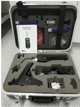
Handheld battery-run portable meter and data logger for the concentration of total VOCs in the air. Limit of detection: 10 ppb, resolution 1 ppb, linear range 10 ppm. ppb RAE – 3000.
