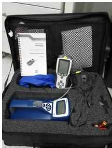
Measurement of ultrafine particulate levels - detection of ultrafine particles smaller than 0.1  $\mu\text{m}$  (or 100 nm). Included Items: telescoping sample probe, sample tube, inlet screen, spare wicks (2), battery holder, and alcohol fill capsule with storage cap, alcohol cartridge, 30ml bottle Reagent Grade Isopropyl alcohol (16), zero filter (2), carrying case, TrakPro software, computer cable, operation and service manual. TSI - P-Trak 8525
