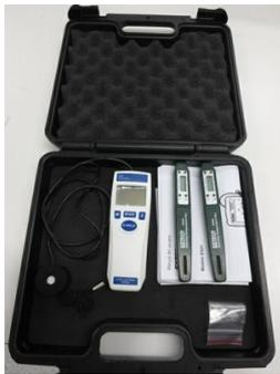
Measurement of damaging UV (long and medium wave UV-A/B) light in the environment and museums.
