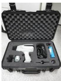
Handheld portable battery-run NIR spectrometer for material identification and characterisation. Equipped with multivariate software and method builder. Sampling spot diameter 5 mm. Polychromix - Phazir
