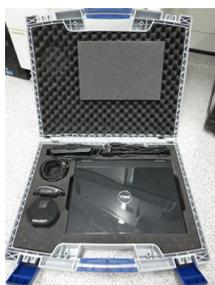
Optical profilometer for assessment of surface roughness, resolution 3  $\mu\text{m}$ , measured area 5x5 mm. Innowep – TraceIT.
