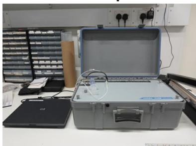
Portable battery-run membrane-introduction mass spectrometer (with no pre-separation of volatiles) for analysis of volatile compounds in air samples. Useful for identification of VOCs in high concentration in a complex matrix or for characterisation of complex mixtures. KORE - MS-200.
