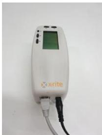
Measurements of density, colour and spectral data. Measurements of light intensity by measuring the wavelength of light. The spectrophotometer will illuminate the sample for measurement with white light. The reflectance of a sample is expressed as a fraction or as a percentage. Selection of measurement aperture - microspot 1.6 x 3.2mm, small 2.0mm, medium 3.4mm or large 6.0mm. X-RITE 500.
