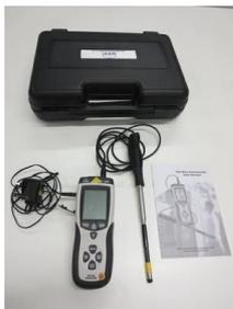
The ATP Hot Wire USB Logging Thermo Anemometer is used for low air velocity (0.1 to 25m/sec) and volume measurement. Measures also temperature and relative humidity. The slim plug in telescopic hot wire probe extends from 0.3 to 1m (including handle). It has a probe sensor head 9mm diameter and has a USB interface for real time transfer of readings to a PC or laptop.
