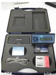
Measurements of gloss using a specialist geometry often specified in the ceramics, metal manufacturing and film making industries. 0.1GU resolution and 0.2% repeatability. Rhpoint Instruments - Novo-Gloss Lite 20°.
