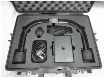
Provides high resolution (16M, 0.05 mm) IR reflectography images of a surface (e.g. a painting), portable, equipped with a macro lens for close-ups. Key features: High resolution images (16 mega pixels). Object resolution down to 0.05mm (0.002 inches). Zoom in and out of the screen to look at fine details. Simple controls allow selection and capture of an area of interest. Fast focus mode allows the
