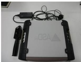
Portable UV-VIS-NIR spectrometer for material identification and characterisation. Equipped with fibre optics sampling accessories to accommodate materials of different size and shape. Sampling spot diameter 2-10 mm. LabSpec – 5000.
