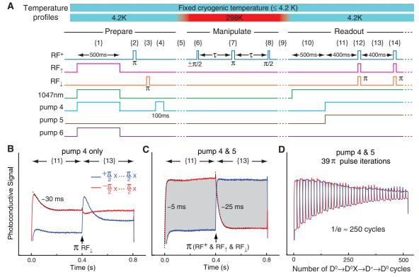
is compared with (C), the improved scheme for D<sup>+</sup> readout (14). The detected signal is proportional to the shaded area. (D) The cycle shown in (C) extended to 39  $\pi$  pulse inversions (16 s).
