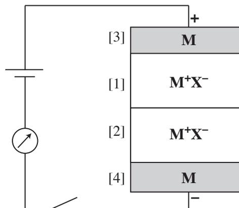
After passing a current of 1 mA for 10 hours, the four pieces are separately weighed. Piece [2] has decreased in mass by 2.2 mg, while [1] has grown by 2.2 mg. Piece [3] has decreased in mass by 8.6 mg while [4] has grown by 8.6 mg. Find the relative contributions of Na<sup>+</sup> and Cl<sup>-</sup> ions to the conductivity.
