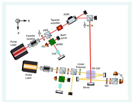
Figure 2 Experimental setup of a radio-frequency atomic magnetometer. From Yao et al. Optics Express 31, 27287 (2023)
