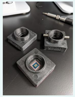
3D printed CCC camera housings
