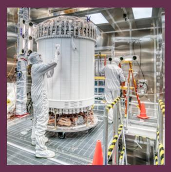
allowed construction of the key background model against which the significance of any possible signal will be evaluated. During the on-site construction of the detector over the last few years, UCL students and post-docs bore key responsibilities, including maintaining strict cleanliness protocols as well as the commissioning of the inner TPC - the very core of the experiment.
