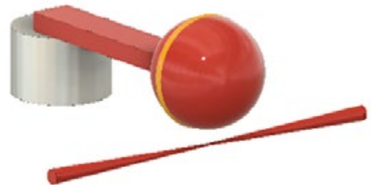
Figure 2. A schematic of the whispering gallery mode acceleration sensor. Light propagating within an optical fibre leaks into the optical whispering gallery mode of the resonator. The amount of light that is coupled into the microsphere is a precise measurement of the separation between the sphere and the optical fibre.
