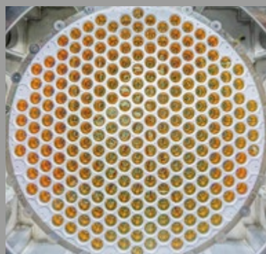
An assembled array (one of two) of 241 ultra-radiopure photomultiplier tubes that will image the liquified xenon target at the heart of the LUX-ZEPLIN experiment.
