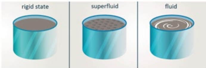
Figure 1. The diagrams illustrate that when the rigid state is rotated it is completely unresponsive, unlike a normal fluid which flows with the rotation and a superfluid which forms quantised vortices.
