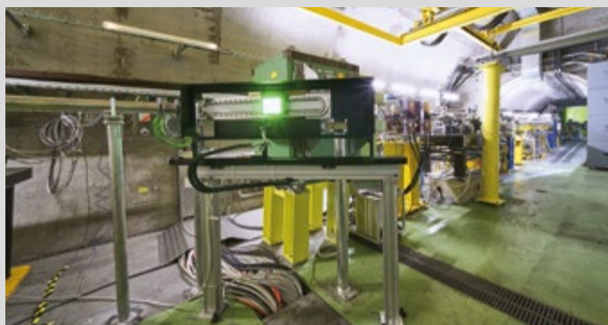
A UCL-built magnetic spectrometer to measure accelerated electrons in AWAKE. Credit: Maximilien Brice, Julien Ordan/CERN
