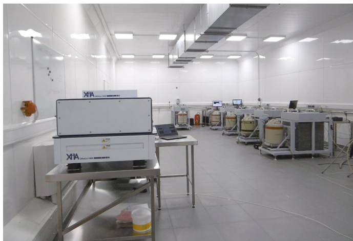
Figure 1 The Boulby Underground Germanium Suite (BUGS) – a state-of-the-art underground facility for measuring ultra low contaminations of radioactive elements in materials.
