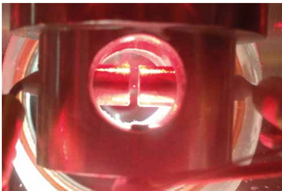
Figure 4. A silica glass sphere held in an ion trap.
