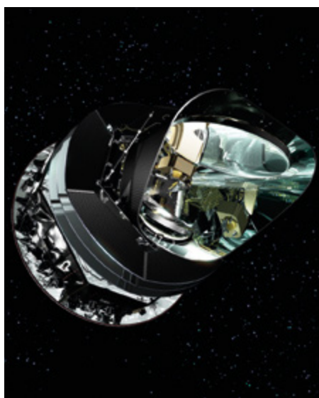
Artist's rendering of the Planck satellite with a view inside the telescope shields. The focal plane unit is visible as the golden collection of waveguide horns at the focus of the telescope positioned inside the thermal shields (external envelope). These protect the telescope from unwanted straylight and aids the cooling of the telescope mirrors by having a black emitting surface on the outside and a reflective one on the inside. For reference, the Earth and Sun would be located far towards the bottom left of this picture.
