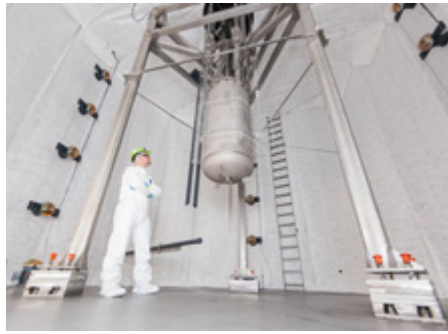
Figure 2. The LUX detector housed in a water tank 1.5 km underground in the Davis Cavern at the Sanford Underground Research Facility. Credit: Matt Kapust, SURF.
