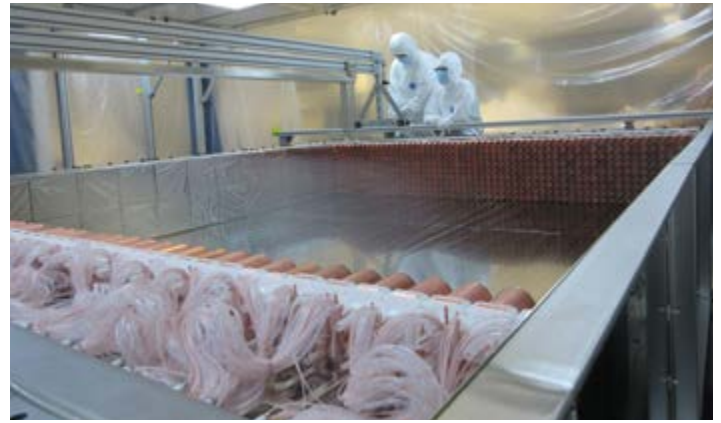
Figure 3. Banks of Geiger cells being inserted into the 3rd SuperNEMO tracking detector module at the Mullard Space Science Laboratory (MSSL) in January 2016. The fourth and final module is scheduled for completion in June 2016, marking the completion of UK construction phase for the project.
