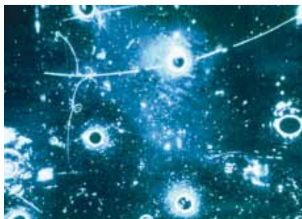
Fig 3. A leptonic weak neutral current event in which the neutrino has scattered off an electron in the heavy liquid by exchanging the Z boson.
