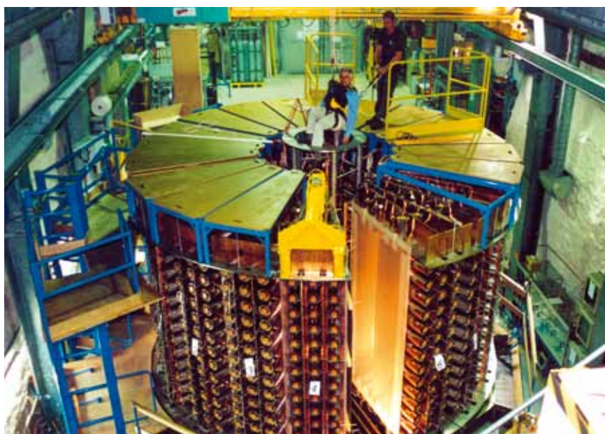
Figure 1: The NEMO 3 detector under construction in the LSM. The figure shows the tracker and the calorimeter arranged together in wedges. UCL takes a leading role in the acquisition and analysis of the data.
