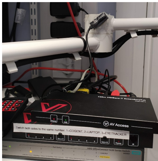
Display switch and remote. Make sure you select the appropriate source to display to your participants in the scanner. Select the same source on the scanner projector (TV1) and the PROJECTOR display in the console room (TV2).
