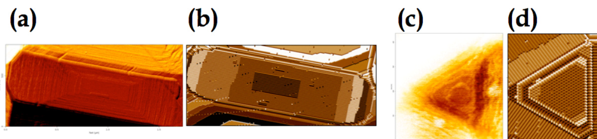
Fig. 2. a) AFM deflection image of a {110} face ( 1 \times 2 \mu\text{m}^2 ) and its simulation image (b). c) AFM lateral force image of a {111} face ( 450 \times 450 \text{nm}^2 ) and its simulation image (d).
