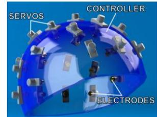
Fig 5. The servo-electrode helmet automatically optimises electrode contact throughout recording period
