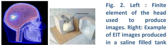
Fig. 2. Left : Finite element of the head used to produce images. Right: Example of EIT images produced in a saline filled tank
