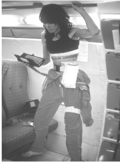
Figure B.6. Miniature Sheffield mark 1 APT system designed for the Juno space mission (courtesy of Prof. B. Brown).
