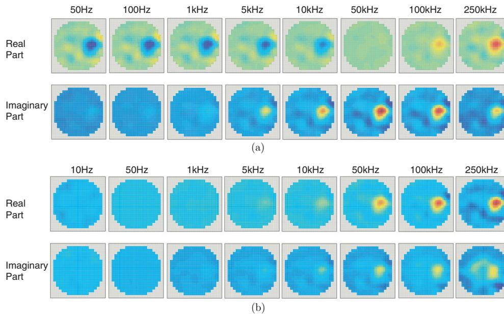
**Figure 8.** (a) Time-difference images of a banana object inside the saline phantom. Reference data were obtained from the homogeneous phantom at each frequency. (b) Frequency-difference images of the same banana object with the data at 100 Hz as the reference data. All images at the same row are displayed with the same scale.
