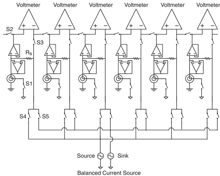
**Figure 4.** A portion of switching circuits on the analog backplane.
