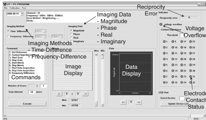
Figure 3. Developed multi-frequency EIT system software.
