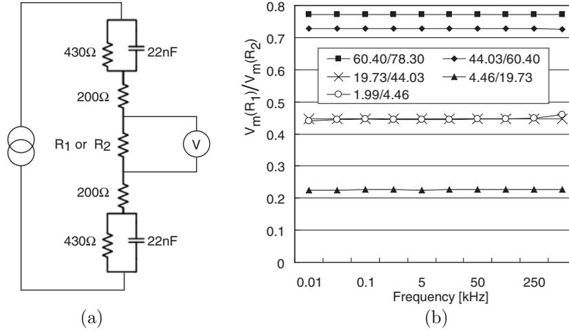
**Figure 7.** (a) Setup for the linearity test using simulated skin impedances. (b) Plots of ratios of measured voltages across two resistors. For example, 60.40/78.30 means that we chose two resistors of  $R_1 = 60.40$  and  $R_2 = 78.30$   $\Omega$  with the ratio of 0.77.
