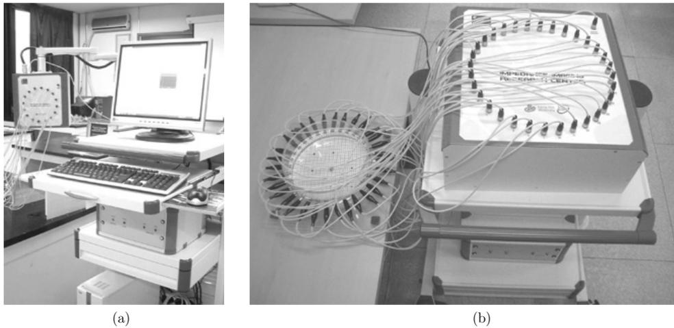
**Figure 1.** Developed multi-frequency KHU Mark1 EIT system. (a) 16-channel and (b) 32-channel.
