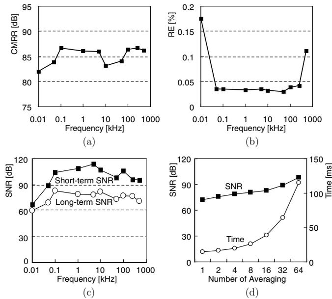
**Figure 6.** Voltmeter performances: (a) CMRR, (b) RE and (c) SNR over the frequency range. (d) SNR at 50 kHz improves as we increase the number of averages. We have to slow down the voltage measurement process to achieve a higher SNR.
