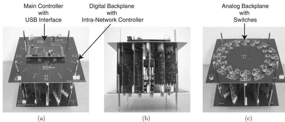
**Figure 2.** Internal views of the developed multi-frequency KHU Mark1 EIT system. (a) Top, (b) side and (c) bottom views.
