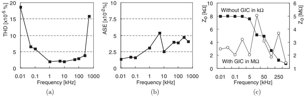
**Figure 5.** (a) Total harmonic distortion (THD), (b) stability error (SE) and (c) output impedance of the current source over the frequency range.
