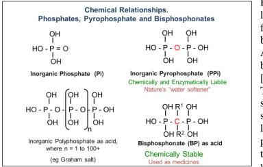
How many of you can look at chemical formulas and not slink beneath your seat? Any unhappy wouldbe chemists out there? [Show of hands] This is actually rather simple. The water softener on the bottom left is just a chain of phosphates joined together with loss of water. Inorganic
