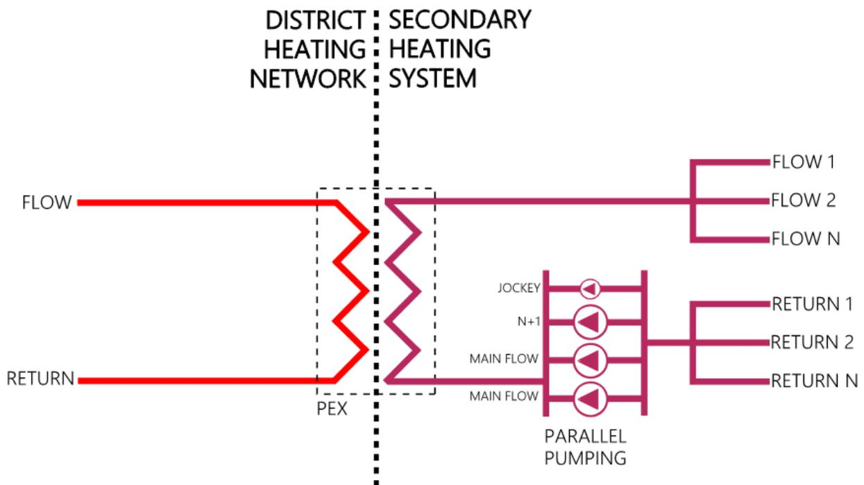
**Figure 8—3 Secondary heat circuit pumping strategy**
