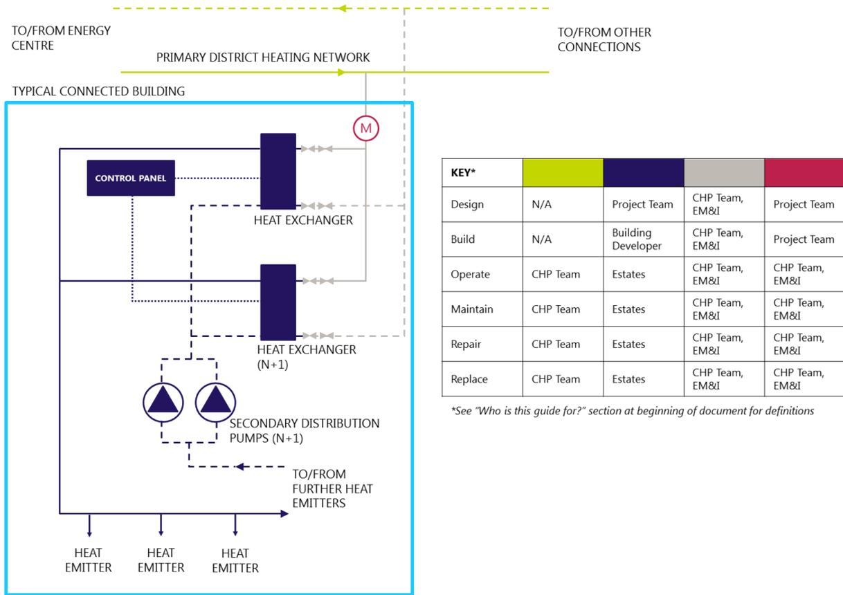
**Figure 6—1 Design, build, operate, maintain, repair and replace responsibilities for district heating network connections**
