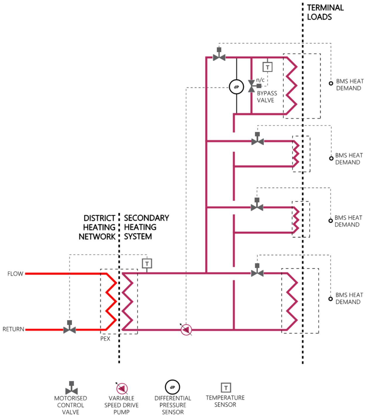
**Figure 8—1 Secondary heating system and connection with district heating network**
