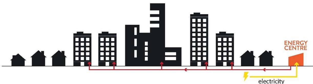
**Figure 4—1 Typical district heating network configuration**
