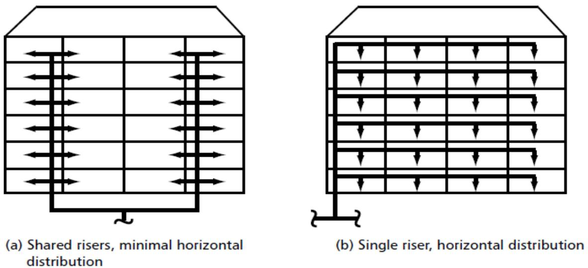
**Figure 8—4 Heat losses reduced in (a) compared to (b) via use of multiple risers, therefore reducing pipe lengths (CIBSE Heat Networks: Code of Practice, 2015)**
