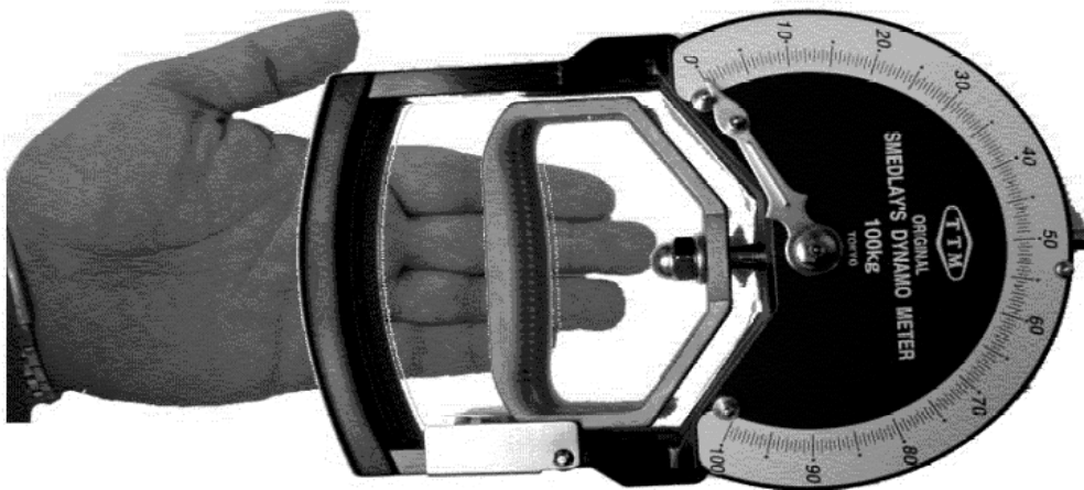
Figure 8 Aligning the dynamometer with the hand
