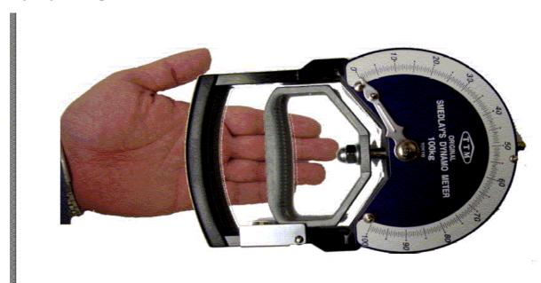
Gripometer lever on second phalanx in gripping action
