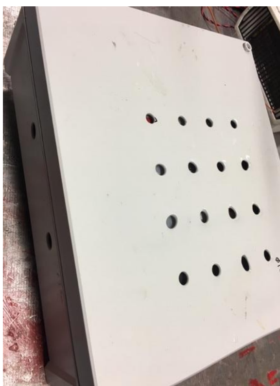
Figure 13. ABS enclosure with the 16 holes drilled on the front and the 2 holes drilled on the sides.
