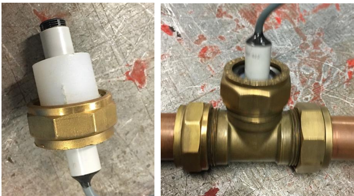
Figure 23. Humidity sensor fitted into copper pipes.
