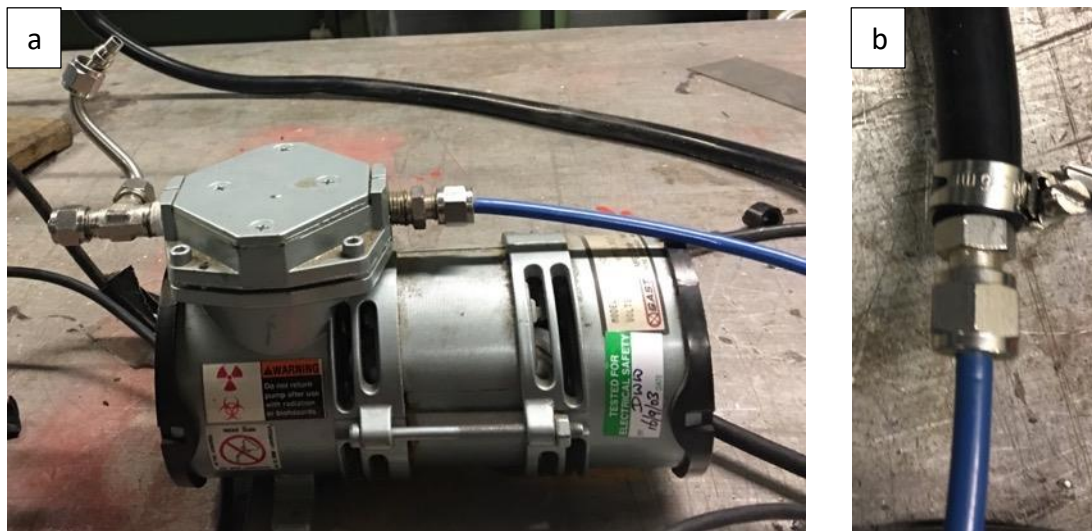
Figure 21. Suction pump used to stimulate air flow through the Econokit device a) connection between suction pump and Econokit set-up b).
