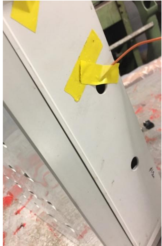
Figure 17. Thermocouple placed inside of ABS enclosure for continuous enclosure temperature readings.
