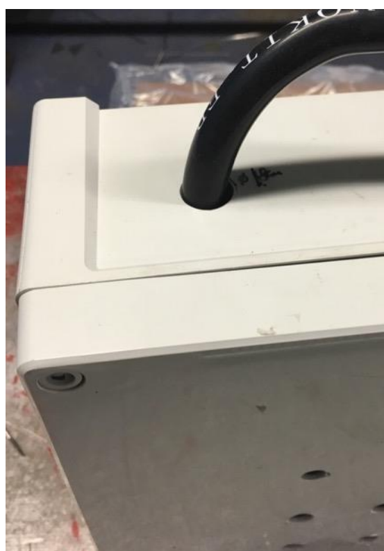
Figure 14. ABS Enclosure with the hole drilled at the top for hose connection.
