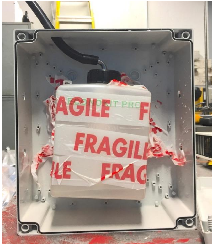
Figure 15. Econokit bubbler fixed in the ABS enclosure with tape.
