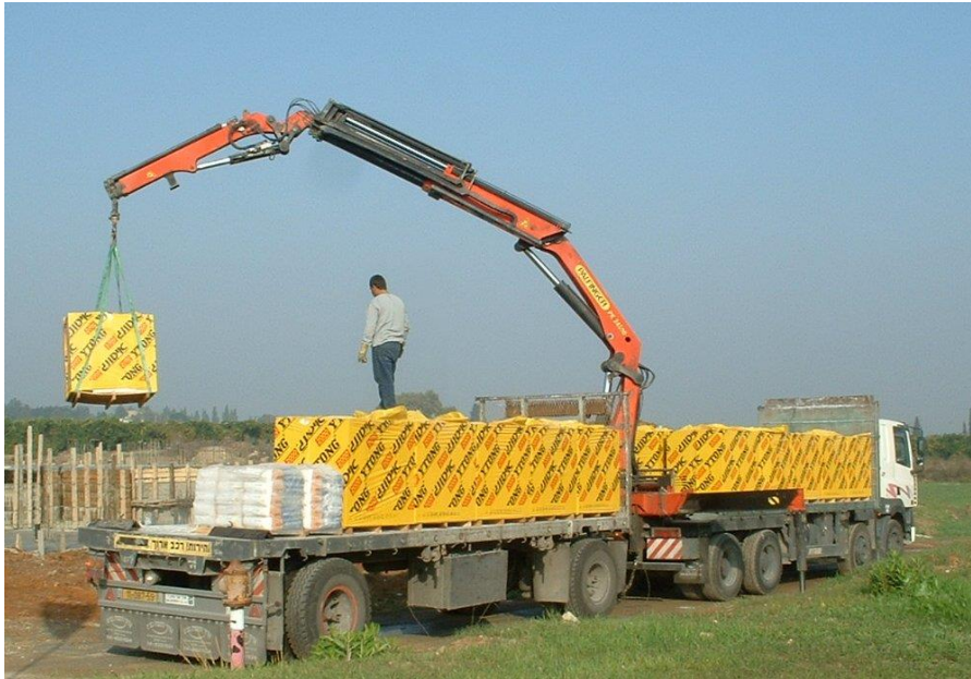
Figure 14: Articulating crane on car (Creative Commons)
