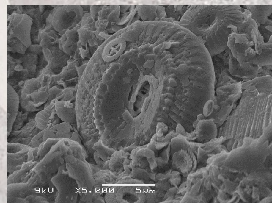
Secondary Electron image of a rock chip showing Coccolithophores of various sizes, (a type of Microfossil) taken on the Departmental JEOL JSM 6480 LV.
