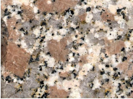
Figure 7 Pink granite, polished slab. The grey crystals are quartz, the white and grey are feldspars, and the black crystals are mica ( UCL Geology Collections)
