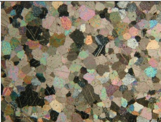
Figure 5 Thin section of a marble viewed between crossed polars. Note the equal sized, interlocking grains (P6149, UCL Geology Collections)
