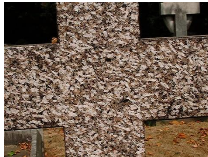
Figure 12 Granite with white feldspar phenocrysts. The rectangular feldspars show some alignment from lower right to top left. This granite was probably quarried in SW England. (City of London Cemetery)
