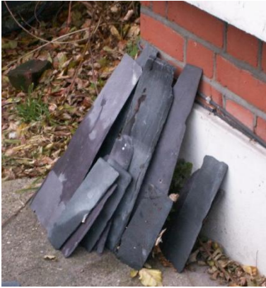
Figure 45 Stack of broken roofing slates, showing slaty cleavage
