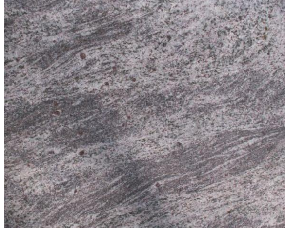
Figure 54 Gneiss showing rounded crystals of reddish garnet (City of London Cemetery)
