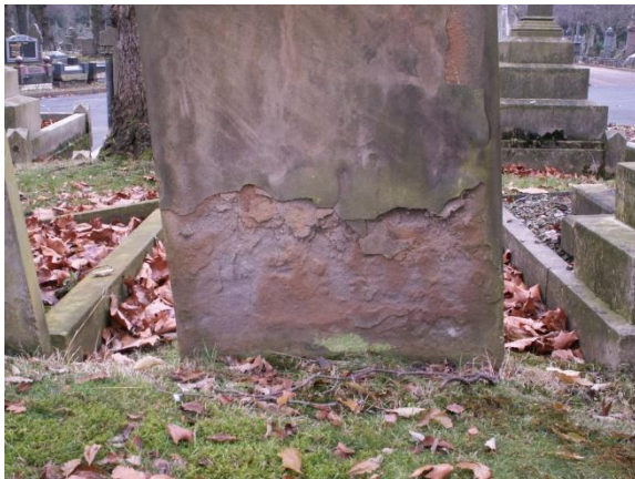
Figure 34 Weathered sandstone; the flaking is particularly pronounced at ground level ( City of London Cemetery)
