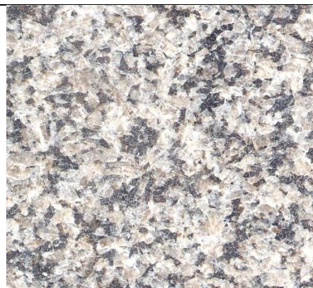
Figure 14 Gabbro, polished block. The feldspars are pale and rectangular (X892, UCL Geology Collections)
