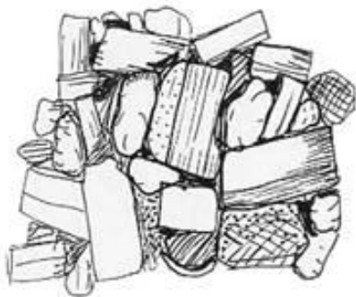
Figure 1 Sketch of granite to show interlocking crystals (courtesy Dr. Eric Robinson)
