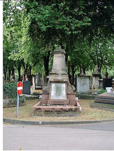
Figure 33 Memorial with red sandstone at the base, and buff coloured sandstone above. The white tablet is made of marble (City of London Cemetery)
