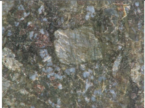
Figure 56 Gneissic rock (originally an igneous rock?). Note the garnets, bluish quartz crystals, and the large feldspars, up to 10cm long. (City of London Cemetery)
