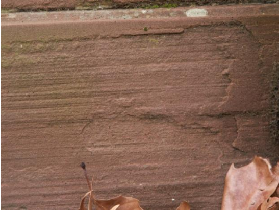
Figure 32 Sandstone showing roughly horizontal lines, which represent bedding.
