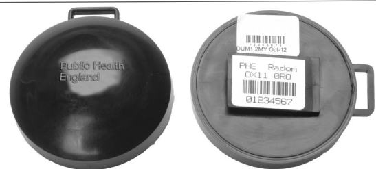
Passive monitors used by Public Health England to measure indoor radon concentrations. Used with permission © Crown Copyright, 2013. Public Health England
