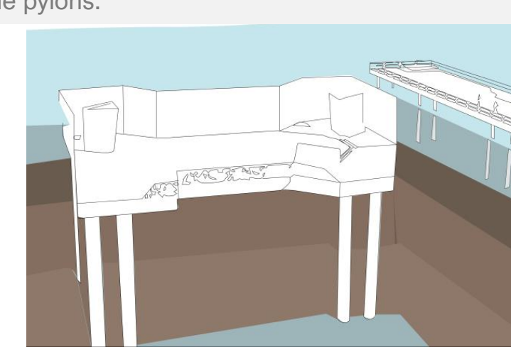
Figure 12: Installation of pile cap
