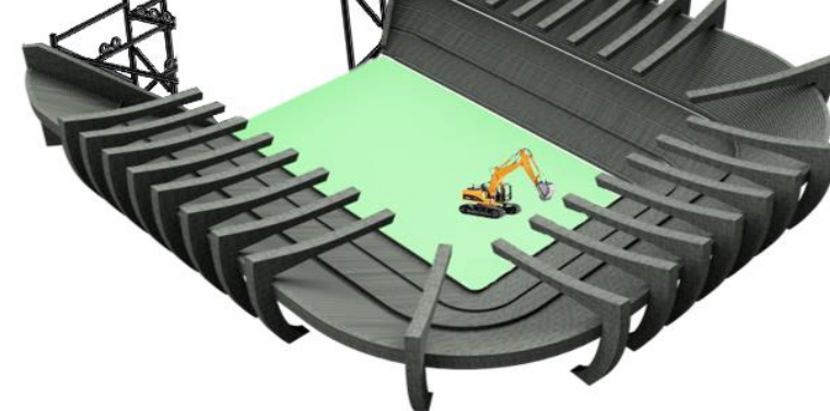
Figure 20. Removal of South Stand for Access to Inner Bowl
