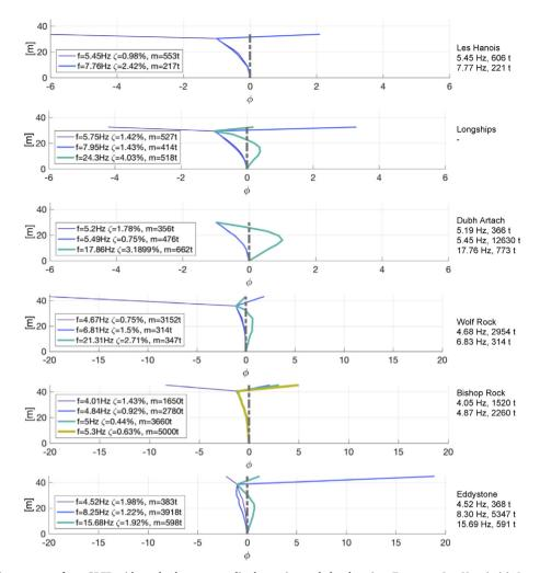
**Fig. 12.** Modal parameters from GRFP with mode shapes normalised to unity at shaker location. From top: Les Hanois (x), Longships (x), Dubh Artach (x), Wolf Rock (x), Bishop Rock (y), Eddystone (x). Frequency and modal mass estimates obtained from measurements in the alternate orthogonal direction are in right hand column.
