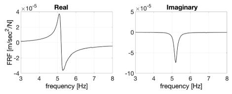
Fig. 11. Real and imaginary parts of FRF for Dubh Artach (y direction).
