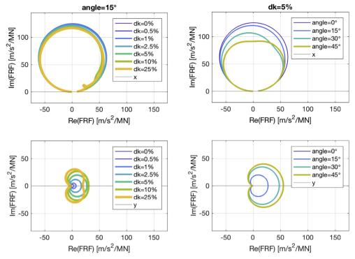
Fig. 14. Nyquist plots for biaxial (x,y) measurement of unidirectional (x) forcing of rotated stiffness system, to same scale. Left:  $\theta = 15^{\circ}$  with increasing stiffness difference. Right 5% stiffness difference with increasing angle. Upper is the direct point mobility FRF, lower is the transverse-mobility FRF.
