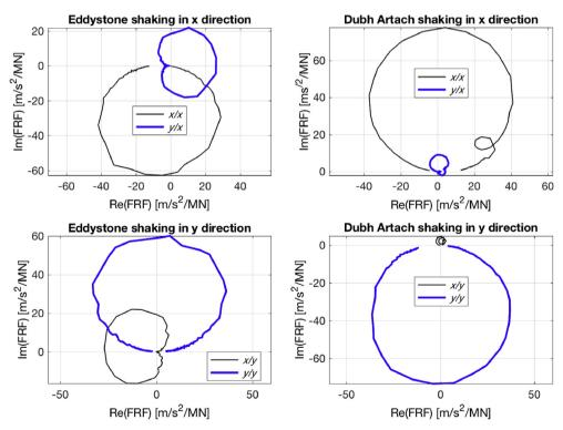
**Fig. 15.** Nyquist plots of point mobility frequency response functions for Eddystone (left) and Dubh Artach (right). Thin line indicates x direction response, thick line indicates FRF for y direction response.
