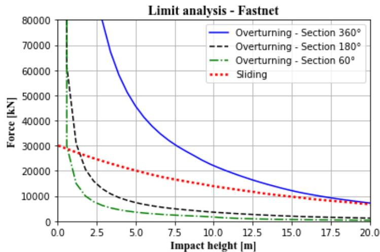
Figure 3. Limit analysis curves for overturning (continuous, dashed and dash-dot lines) and sliding (dotted line)
