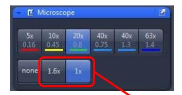
5x, 10x 20x & 40x dry objectives. The last two (40x 1.3 & 63x 1.4) are oil objectives.
