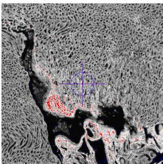
Reset the Display histogram, then adjust the bulb power and exposure time to approximately half fill the histogram, and avoid any saturated pixels.
