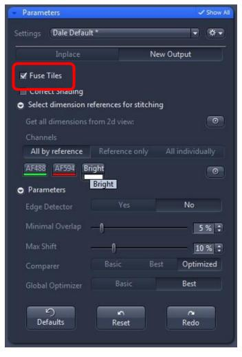
By default it will use the first channel captured to align the image, (normally Dapi) but you can choose any channel that has sufficient content to perform the stitching.
