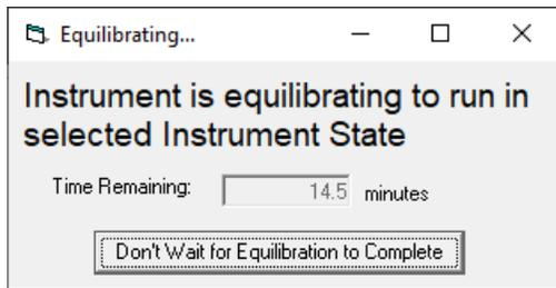
Figure 2 Instrument equilibrating after changing mass range.
