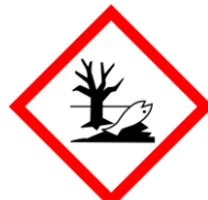
Dangerous to the environment
