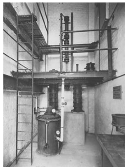
Bubble cap distillation column in the Ramsay Laboratory, 1931
