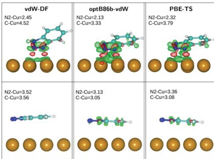
Fig. 2 Electron density difference plots for the 'Tilted' (top row) and 'Flat' (bottom row) BTAH/Cu structures using three representative vdW-inclusive functionals. Green represents the region of charge density depletion and red regions of accumulation. The iso-surface level is  $0.002e/a_0^3$  for all structures. The distance between the azole N2 and the surface and between the centre of the benzene-like ring and the surface are given in Å.
