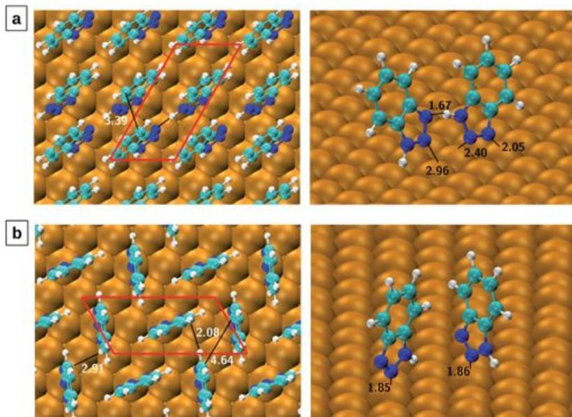
Fig. 4 Top (left-hand-side) and side (right-hand-side) views of the most stable structures for BTAAH at 1/4 ML coverage (a) HB dimer structure. (b) Non-HB upright structure. The red box shows the unit cell. Selected distances are shown in Å. In the top views the unit cell and periodic replicas are shown. In the side view only the molecules in the unit cell are shown for clarity.
