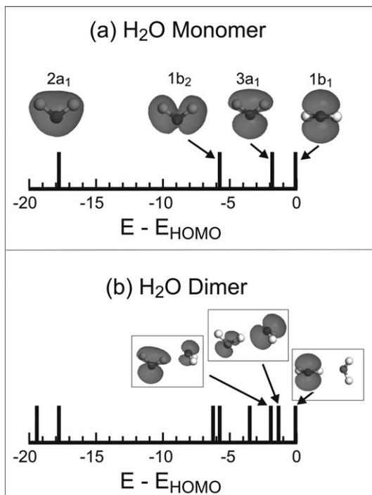
**Fig. 5** DFT computed energy level diagrams and selected Kohn–Sham orbitals for the highest occupied orbitals of an isolated (gas phase) H<sub>2</sub>O monomer (a) and an isolated (gas phase) H<sub>2</sub>O dimer (b). The energy of the highest occupied molecular orbital ( $E_{\text{HOMO}}$ ) is set to zero eV in each system.
