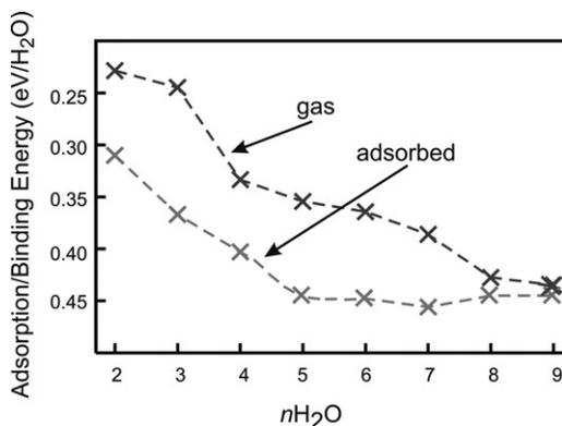
**Fig. 4** Plot of the adsorption energies and binding energies for adsorbed  $n\text{H}_2\text{O}$  ( $n = 2\text{--}9$ ) clusters on Cu(111) and for gas phase  $n\text{H}_2\text{O}$  ( $n = 2\text{--}9$ ) clusters. The structures of the 7–9 H<sub>2</sub>O molecule gas phase and adsorbed clusters are taken from ref. 45 and ref. 35, respectively. The dashed lines are merely guides to the eye.
