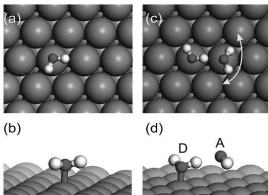
**Fig. 1** Top and side views of the lowest energy adsorbed H<sub>2</sub>O monomer and H<sub>2</sub>O dimer structures identified. In (d) the H<sub>2</sub>O molecule which donates (accepts) the H bond is labelled D (A), and in (c) the arrow is to illustrate that rotation of the acceptor H<sub>2</sub>O in a plane about the surface normal is facile.
