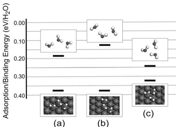
**Fig. 2** Relative energies and structures of three gas phase and adsorbed H<sub>2</sub>O trimers. Adsorption energies and binding energies are relative to isolated gas phase H<sub>2</sub>O molecules as defined in eqn (1) and (2), respectively.
