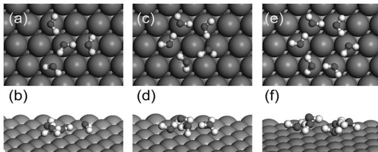
**Fig. 3** Top and side views of the lowest energy structures identified for an adsorbed H<sub>2</sub>O tetramer ((a)–(b)), pentamer ((c)–(d)), and hexamer ((e)–(f)) on Cu(111).
